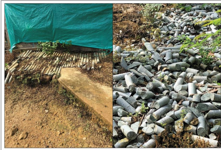
Figure 4-6: Core either abandoned or used as construction materials for sidewalk (path)
